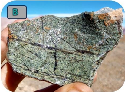
RC21930, Quartz veinlets in sericite alt diorite. Au: 0.50 g/t, Ag: 0.3 g/t, Cu: 356 ppm, Mo: 9.2 ppm
