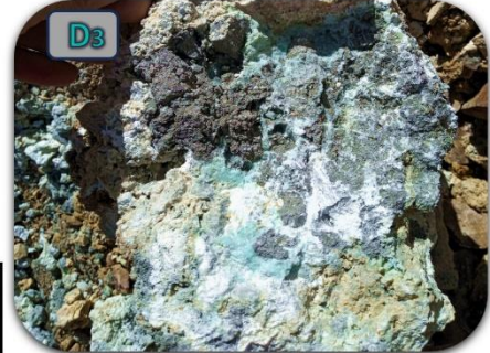
RC21902, select sample of Pyrite – energite + copper oxides from structure in D1 Au: 0.97 g/t, Ag: 14.7 g/t, Cu: 0.36%, Mo: 5.9ppm
