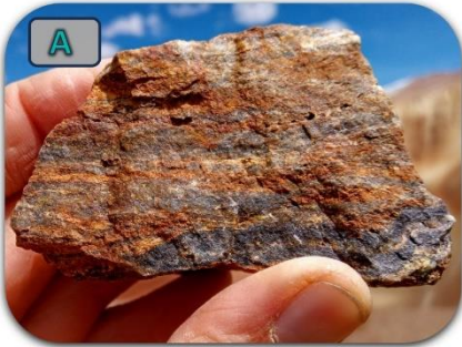
RC21893, Quartz veinlets ± sul. Au: 0.75 g/t, Ag 1.3 g/t, Cu: 354 ppm, Mo: 41.8 ppm
