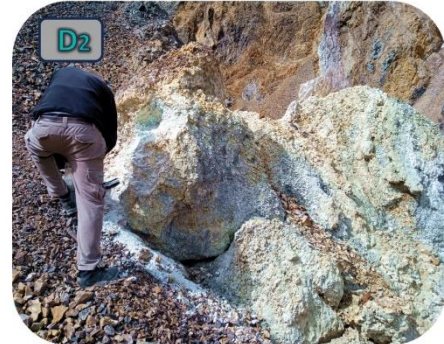
RC21903, channel sampling of 6m-wide structure with adv. Argillic alteration. Pyrite, energite, copper oxides 1m channel sample at 0.53 g/t Au, 17.5 g/t Ag, 861ppm Cu, 6.8ppm Mo
